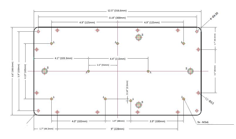
\*NOTE: The threaded inserts labeled "B" in the above graphic are 1/4"-20TPI and are meant to be used with I-beam clamps for easy mounting to the I-beams
